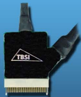
32 Ch headstage amplifier with 3 wires
