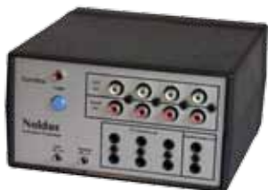
The front of the SyncBox, with sockets for a variety of signals.
