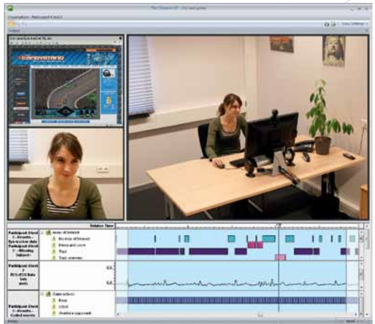
A multi-modal recording in The Observer XT. It contains a screen capture video, a camera image showing a user close-up, a dome camera overview, manually recorded behavior, eye tracking data, and an ECG signal.
