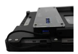
MATERIALS Aluminium materials with black microtexturized electrostatic paint finish, translucent acrylic and PLA printed components. DIMENSIONS 24 high, 34 long, 4 width **PORTS** 3 hub 250 mA enabled for connecting elements such as a mouse, keyboard, SPEED Minimum 1ms of precision COMPATIBILITY USB 3.0 Compatible
