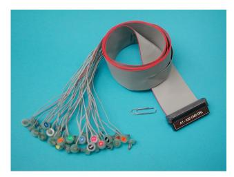
The BioSemi "Pin-type" Active electrode has been designed especially for mounting in BioSemi headcap's. The electrode has a sintered Ag-AgCl electrode tip, providing very low noise, low offset voltages and very stable DC performance.
